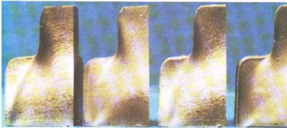
Plate 2. Shear bands are evident on the plane normal to the ram along the axis of the bar-stock
